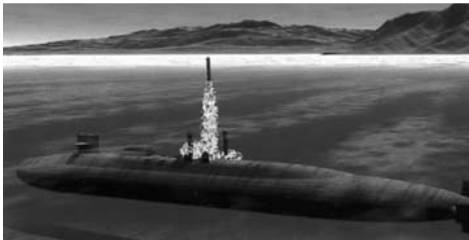
Figure 1. An artist's concept of a Trident-class SSGN firing a Tomahawk cruise missile, with an Advanced SEAL Delivery System locked onto the submarine's forward missile tube
