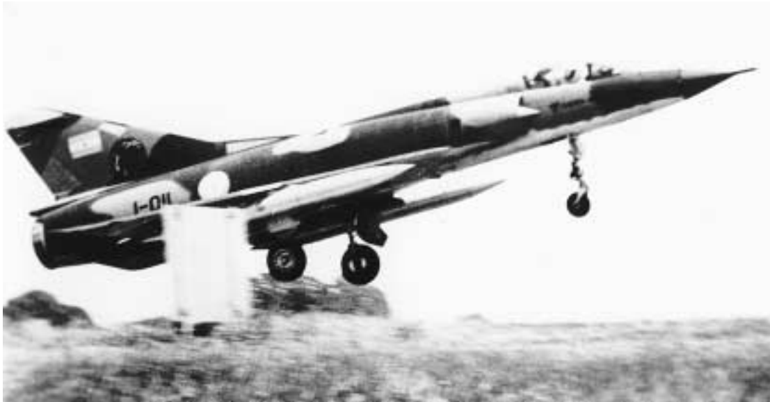
The FAA's Dassault Mirage III interceptors were the equal of most of the world's frontline aircraft but were severely limited in air-to-air combat by their primary air intercept missile—the French-made infrared Matra 530.
